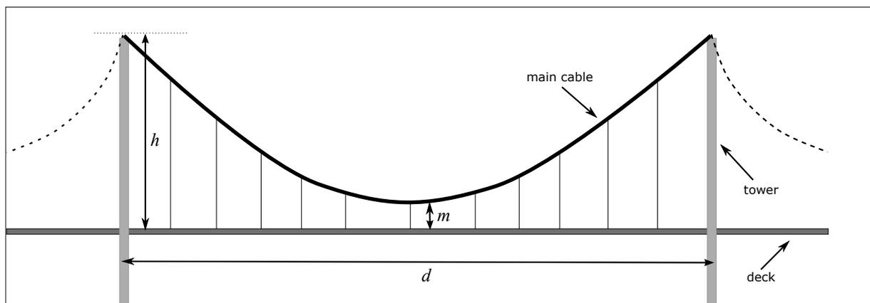
Figure 1: Diagram of a suspended deck bridge
